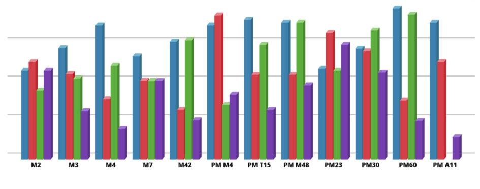
Wear Resistance 📕 Toughness 📕 Red Hardness 📕 Ease of Grinding
